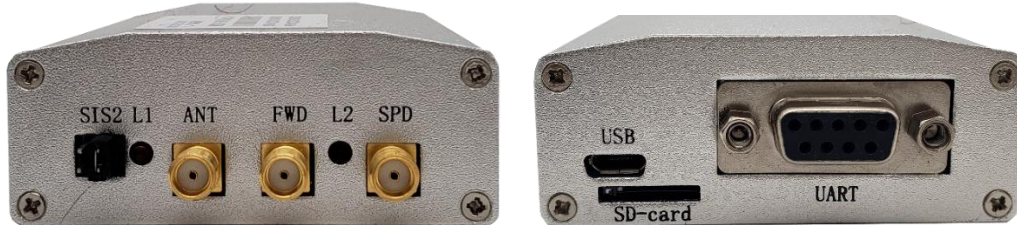
Figure 3-1 Interfaces & Indicators on UM220-INS EVK
