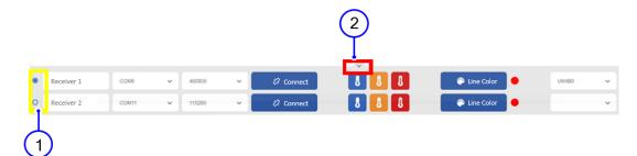
Figure 2-4 Status bar showing all the connected receivers
