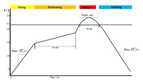
Figure 4-1 Soldering Temperature (Lead-free)
