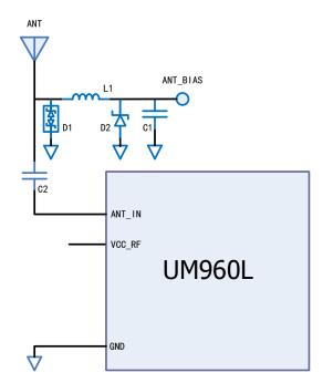
Figure 3-1 UM960L External Antenna Feed Reference Circuit
