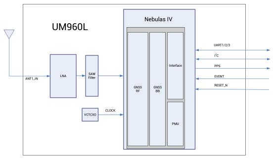
Figure 1-2 UM960L Block Diagram
