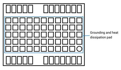
Figure 3-2 Grounding and Heat Dissipation Pad
