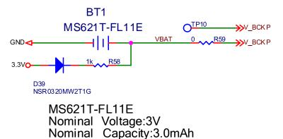
Figure 3-5 Backup Power Circuit
