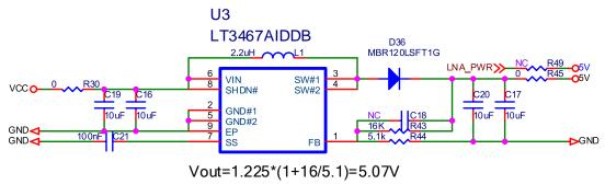
Figure 3-4 5 V DC/DC Boost Circuit
