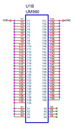
Figure 6-3 Pads (Y1-Y55) and Socket Mounting Holes (X1-X8)
