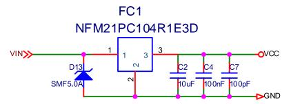
Figure 3-1 Power Filter Circuit
