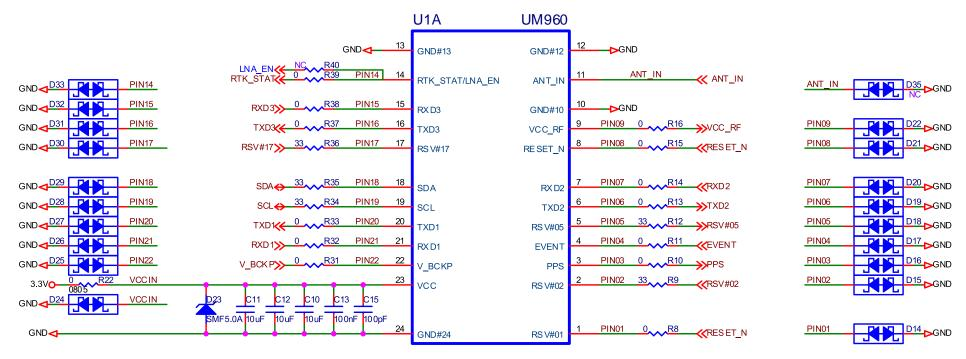
Figure 6-1 UM960 Peripheral Design
