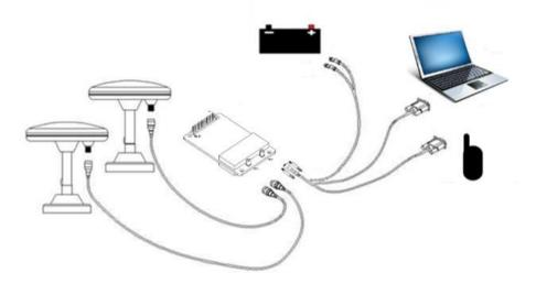
Figure 4-1 Typical Installation of UM482
