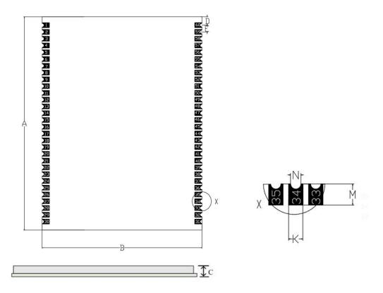
Figure 2-1 UM482 Mechanical Diagram
