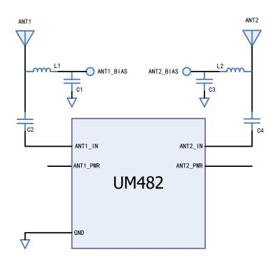
Figure 3-5 UM482 External Antenna Feed Reference Circuit
