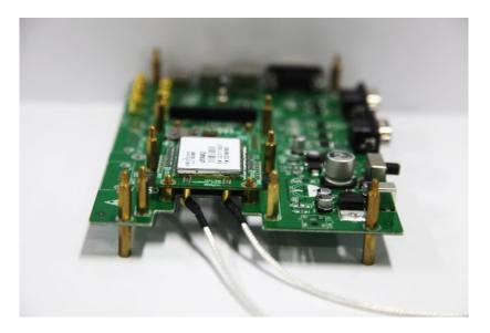
Figure 4-3 Connect the Antenna
