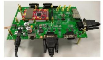
Figure 4-3 UB482 Serial Port, Power Connection
