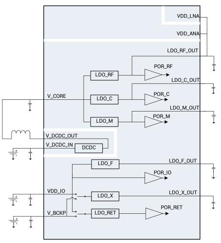
Figure 5-1 DC/DC power-on and sequence
