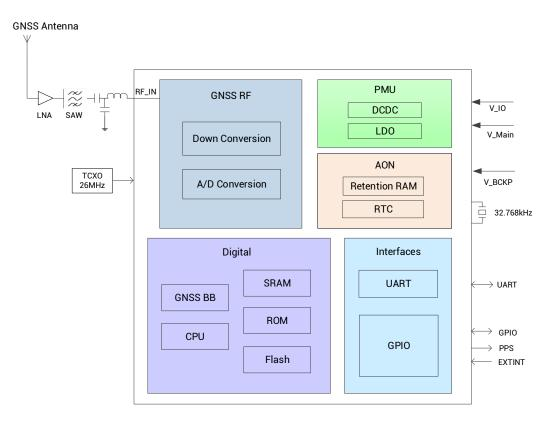
Figure 1-2 UC6226 chip block diagram
