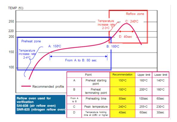
Figure 10-1 Reflow Soldering Temperature Curve
