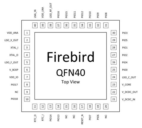
Figure 6-1 QFN40 pin diagram
