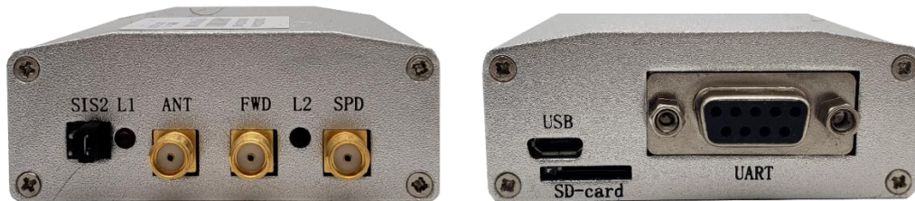
Figure 3-1 Interfaces & Indicators on UM220-IV N EVK
