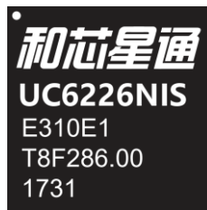
Figure 11-1 QFN product appearance
